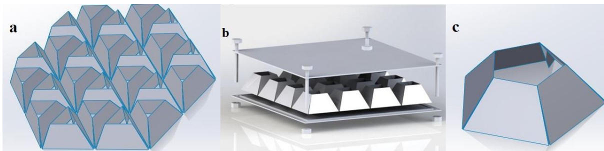
Figure 1: (a) truncated triangular pyramid folded core for cladding; (b) assembling method for quick onsite deployment; (c) single unit cell of truncated pentagonal pyramid folded structure
